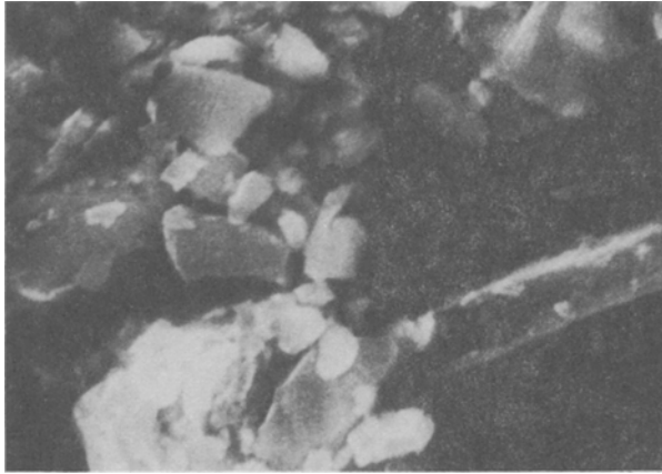
Photo 2 Calcium orthosilicate precipitations in the vicinity of the ferrites of ternary system in the 1.9 basicity sinter. Scanning electron microscope, 4600×
